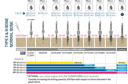
IMPORTANT: control the drilling axis by applying intermittent (tapping) pressure, always in the vertical plane, taking care not to exert excessive pressure on the bone
