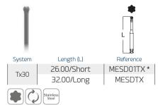
Do not exceed 30 Ncm as it could cause severe damage to the screwdriver and screw.
