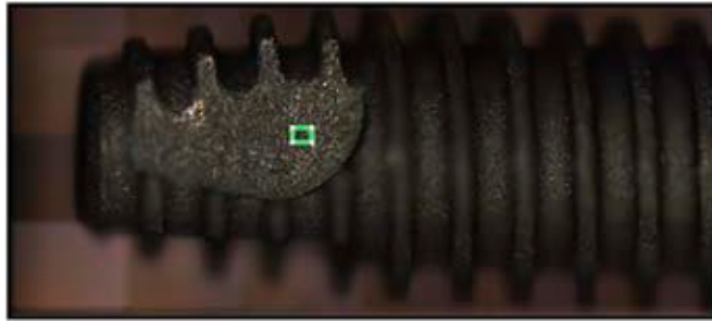
Figure 2. Selected zone for roughness measurement at the apical third of the implant.
